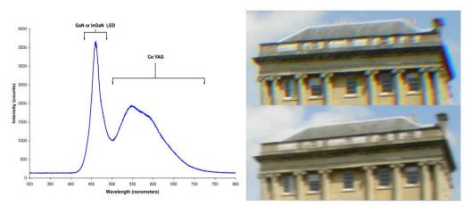
Figure 4. White-led illumination spectrum<sup>5</sup> (left); displayed image without correction<sup>7</sup> (top right); displayed image with correction (bottom right).
