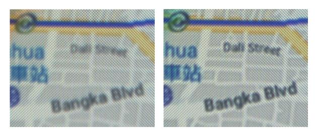
Figure 11. Piece of city map (FOV center): Vive Pro built-in correction (left) and with DL element (right).
