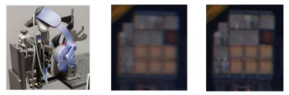
Figure 1. The Digital Lens element reliably improves the image quality of design-constrained near-eye display optical systems. From left to right: Vive Pro Eye HMD mounted for the optical measurements, displayed image with built-in correction, displayed image pre-corrected with the Digital Lens element.
