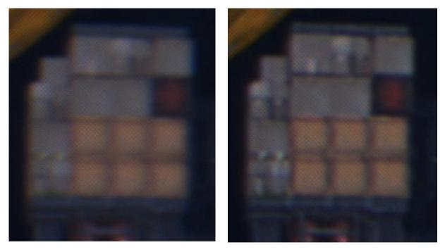
Figure 10. Scene from 'The Lab' VR game (10 degree to the right of FOV center): Vive Pro built-in correction (left) and with DL element (right).
