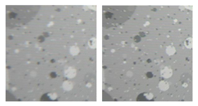
Figure 9. 'Dead leaves' pattern at 20 degree off-center: Vive Pro built-in correction (left) and with DL element (right).
