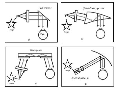
Figure 2. OST-HMD types: Half-mirror (i.e. semitransparent flat mirror or cubic prism) (a.), the Prism-based (b.), the Waveguide-based (c.), and the Retinal Scanning (d.).
