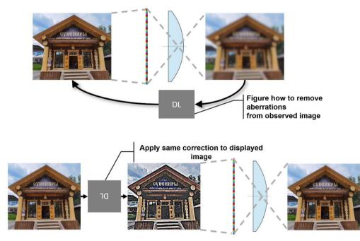
Figure 6. Schematic depiction of aberration correction method
